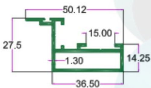
SEC. NO. 2448A (L) WT. 2.820 TO 3.000 KG/15' (H) WT. 3.120 TO 3.250 KG/15'
